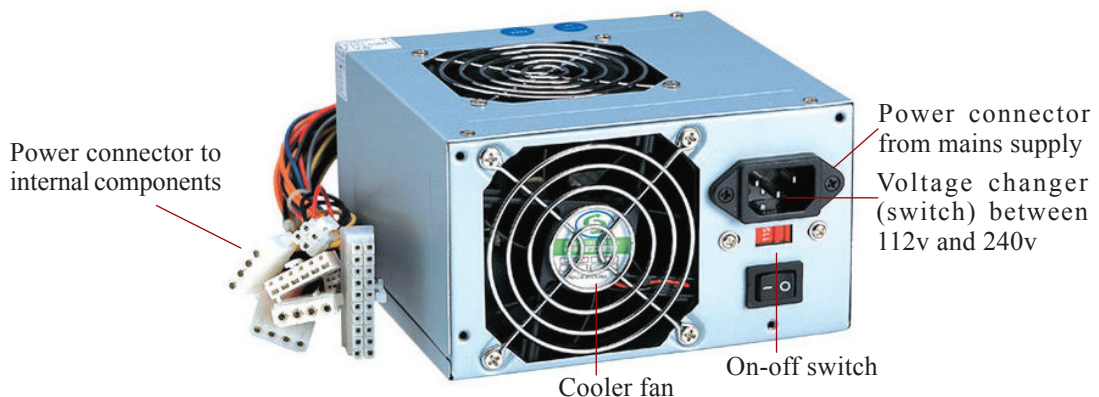
Fig.2.17: Power supply unit.
