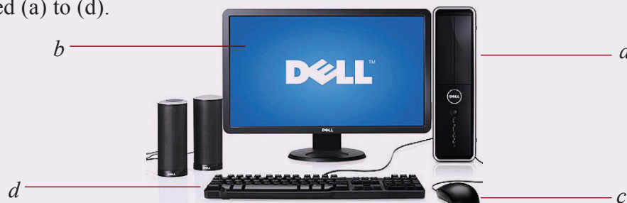
Fig. 1.1: Parts of a computer
