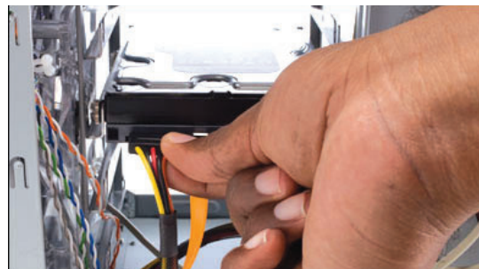
Fig. 2.30: Mounting a hard disk
