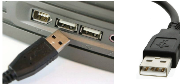
Fig.2.8: USB port and connector
